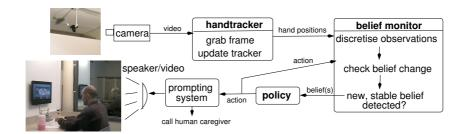
Fig. 1. Schematic of the system with images of test washroom.
