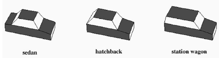
**Fig. 1.** Generic 3D-polyhedral vehicle models without wheelarches. A pixel will be taken into account for vehicle color determination only if this pixel is covered by one of the facets marked in dark gray.
