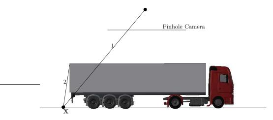
Fig. 4. The bird's-eye view system. First, pixels of the resulting virtual image are projected onto the ground plane and then they are projected to omnidirectional images where the pixel values are constructed by bilinear interpolation.
