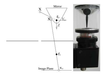
**Fig. 2.** The figure shows the omnidirectional projection. The point **X** is given in the coordinate system defined by the focal point  $\mathbf{f}_0$  within the mirror. The z-axis points towards the image plane.  $\mathbf{f}_1$  is the second focal point with coordinates  $(0, 0, 2c)^T$ . Right: Omnidirectional camera consisting of a hyperbolic mirror with a standard pinhole camera. The black needle in the middle avoids reflections on the glass cylinder [10].
