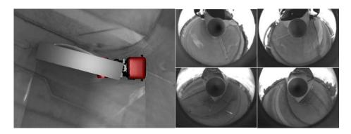
**Fig. 3.** Left: The bird's-eye view image. The kink angle between truck and trailer is  $-14^{\circ}$ . Right: raw images from the omnidirectional cameras.
