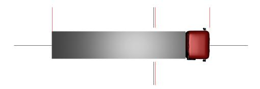
Fig. 5. Several subdivisions to construct bird's-eye view images. The black lines show the division into the cells of points closer to each camera than to any other camera with the exception of the the front and back camera separation line, which is set more to the front to the account for the height of the back cameras. The red lines show the subdivision that removes the most important blind spots. However, there is still a blind volume in the middle part between truck and trailer.
