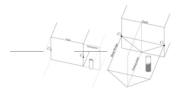
**Fig. 7.** Left: Splitting the space along the baseline of the cameras  $C_1$  and  $C_2$ . Camera  $C_1$  sees the black part of the cylinder and camera  $C_2$  sees the white part. There is no blind spot. Right: Splitting plane along the line of lateral symmetry of the truck. Everything that is within the blind wedge is not seen in the compound image. Thus, the empty part of the cylinder is not seen on the display (See also Figure 6).
