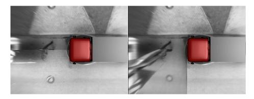
Fig. 6. Left: Bird's-eye view image of the front cameras with a symmetric subdivision along the line of lateral symmetry. The person in the middle of the truck is not fully visible in the resulting image. Right: A subdivision chosen in such a way that the person is always visible in the bird's-eye view image.
