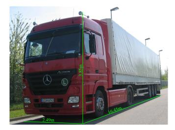
Fig. 1. Mercedes-Benz Actros. The front omnidirectional cameras are mounted below the side mirrors. The back cameras are placed at the top of the trailer.
