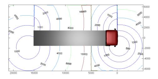
Fig. 8. The resolution of the bird's-eye view system. The Figure shows the contours of a three-dimensional function consisting of x,y coordinates and the area covered by backprojected pixel of the omnidirectional cameras. The values within the plot are the area covered by a backprojected pixel. All values are given in  $mm^2$ .
