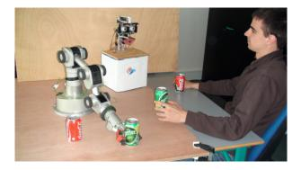
Figure 1: Example of the robotic devices used in our experiments. A 6 DOF robotic arm is used in conjunction with a robotic head for visual perception and interaction.
