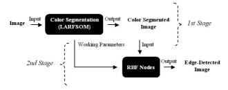
Figure 2 - Proposed two-stage edge detection algorithm.
