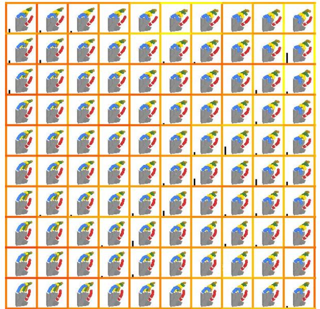
Figure 7: 10x10 extract of the cylinder-specific 25x25 SOM *Grasp Manifold* used for Fig. 3 and Fig. 4 after resuming the learning with grasp postures generated by the experience-based grasp control. The node structure is now very smooth, the hand postures fade smoothly from one node to the next.
