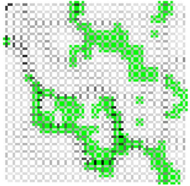
Figure 6: Visualisation of the inter-node distances and the data-projection-nodes of the 25x25 cylinder-SOM. Depicted is Fig. 4a extended by the node matches (green background) when projecting all successful grasp postures from evaluation (force closure grasps characterised by non-zero positive magnitudes of the worst-case disturbance wrench within the L1 grasp wrench space, cf. [3]). The grasp postures match mainly on the inter-cluster nodes.
