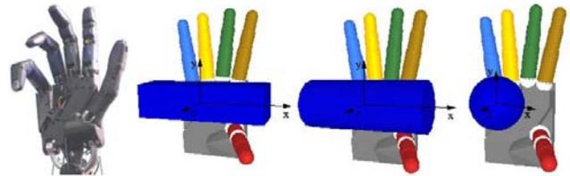
Figure 1: The Shadow Dextrous Hand and its virtual simulation model. Depicted is the initial hand posture with the three studied grasp objects: 1) box ( $4 \times 4 \times 16$  cm), 2) cylinder (l: 16 cm,  $\varnothing$ : 6 cm), and 3) sphere ( $\varnothing$ : 6 cm).
