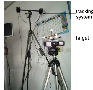
Fig. 4. Tracking system which determines the position of the camera within a global world coordinate system. The camera is labelled with a target.
