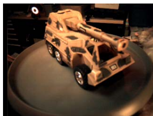
Fig. 2. One of 591 images of a toy artillery piece on a turntable. The average rotation between images is a little less than 1.5^\circ .
