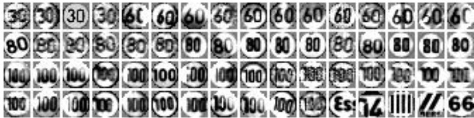
Fig. 5. Typical samples correctly classified by the classifier trained with real samples and incorrectly classified by the classifier trained with synthetically generated samples.
