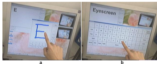
Fig. 6. (a) “E” is written and recognized; (b) “n” key of the keyboard is pressed
