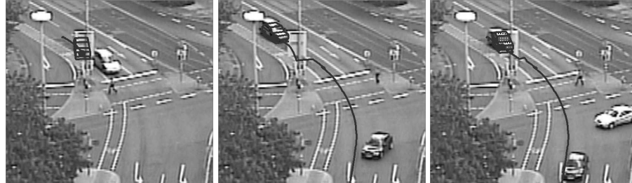
Fig. 2. Tracking of a vehicle which becomes occluded by a traffic sign (left panel: without occlusion detection; center panel: with occlusion detection and motion -based prediction; right panel: with occlusion detection and behavior -based prediction). See Section 5 for further discussion.
