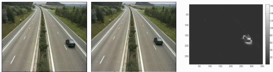
Fig. 2. Two adjacent frames and their intensity difference
