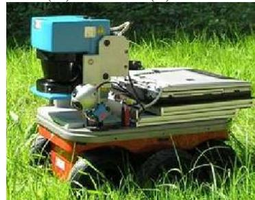
**Fig. 7:** The mobile robot Kurt3D.
