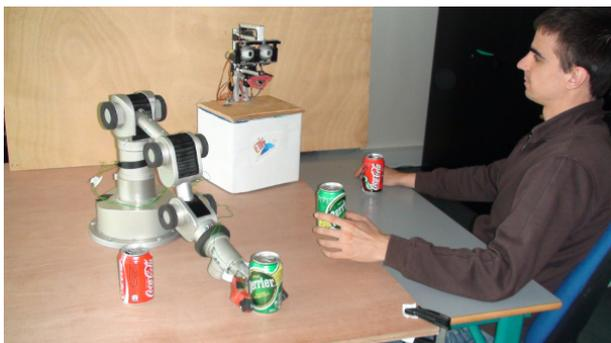
Figure 1: Example of the robotic devices used in our experiments. A 6 DOF robotic arm is used in conjunction with a robotic head for visual perception and interaction.
