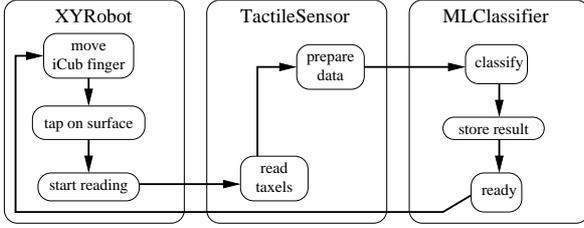
Figure 3: Interaction of modules in the experimental setup. Modules developed with C/C++ and YARP library to a straightforward implementation on the iCub humanoid.
