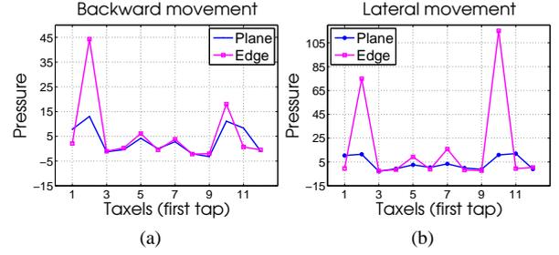
Figure 4: Pressure contact of first tap over plane and edge; (a) backward movement, (b) lateral movement.
