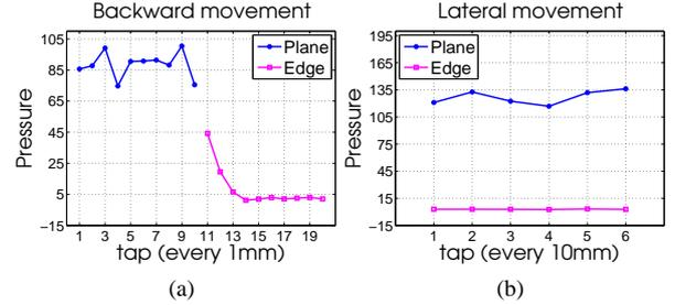
Figure 5: Edge and plane detection in testing phase; (a) backward movement, (b) lateral movement.
