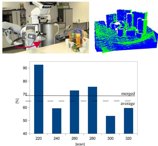
Figure 1: As the camera is moved (left), multiple frames can be captured that cover different parts of the objects in the scene (right), increasing the overall classification accuracy (bottom).
