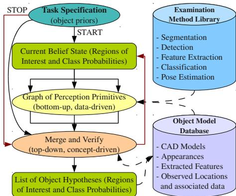
Figure 2: Basic setup of the proposed system for iterative refinement of object hypotheses by multiple methods according to a task specification.
