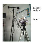
Fig. 4. Tracking system which determines the position of the camera within a global world coordinate system. The camera is labelled with a target.
