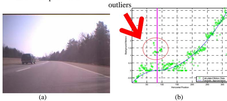
**Fig. 3.** A background motion model. (a) is an original image  $N$ , (b) Illustration of background motion model.
