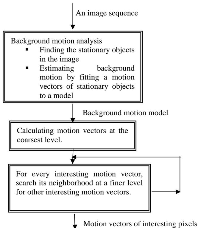
**Fig. 1:** An efficient and effective system for motion vector calculation.
