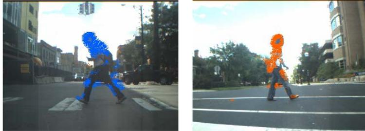
Fig. 6. Two more images showing the motion vectors generated by the proposed system.
