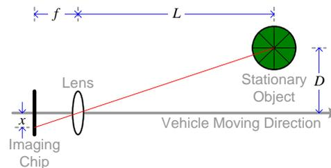
**Fig. 2.** Schematic drawing of background motion geometry.
