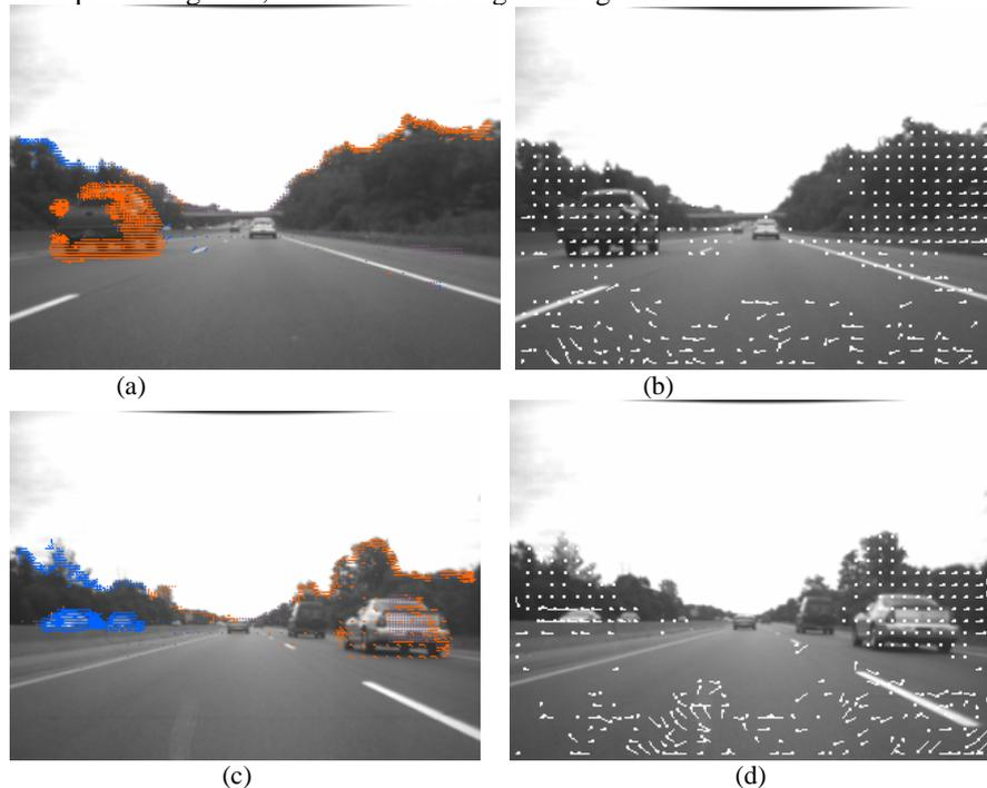
**Fig. 5.** Two examples of motion vector images generated by the proposed algorithm and by a standard SSD based method. (a) and (c) show the motion vectors generated by the proposed system on Image 1 and 2. (b) and (d) show the motion vectors generated by a SSD based correlation method on the same two images.
