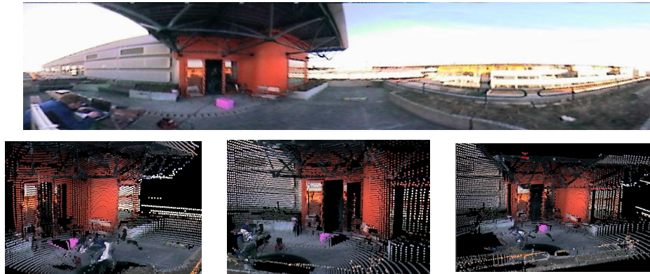
Fig. 8. The panoramic picture shown in the upper window was taken by using a hyperbolic mirror and a perspective camera the size of 640x480 pixels. After calibration, the color information was mapped onto the 3D points extracted by a rotating sick laser range finder. In the lower windows are the results of the mapping. The colors are well reprojected onto the 3D structure of the environment, showing that the camera calibration was accurately done.
