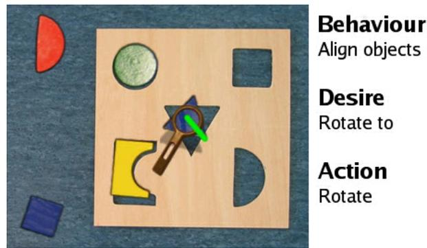
**Fig. 1.** An early version of the COSPAL system solving a simulated shape-sorter puzzle.
