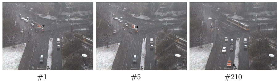
Fig. 2. Car tracking with on-line learning on noisy images
