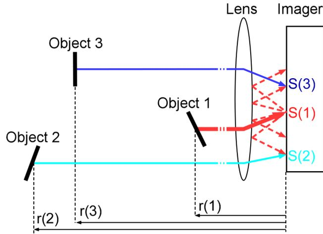
Fig. 3: Light scattering in TOF camera (after [4]).
