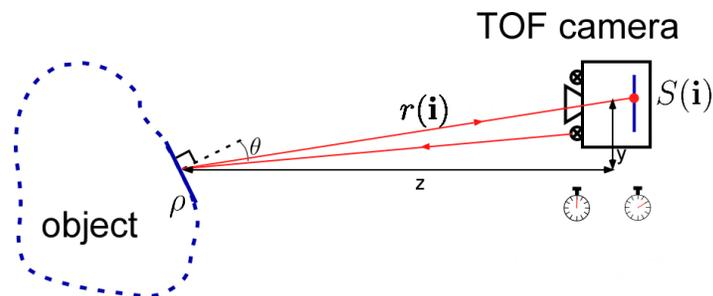
Fig. 1: Time-of-flight camera - Principle of operation
