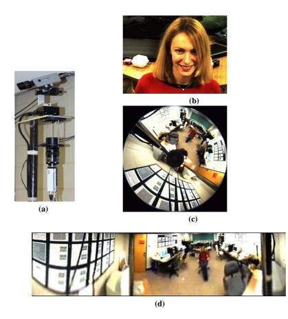
Fig. 1. (a) Foveated panoramic sensor. (b) Raw foveal image. (c) Raw panoramic image. (d) Warped panoramic image.
