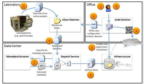
Figure 1: The data acquisition workflow in the nanomaterials lab with the underlying eSciDoc data infrastructure and the eLab Solution to configure experiments and access the gathered data objects.
