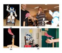
Figure 1: Setup for our experiments. (a) Nao robot (b) Basic Automata (made in the lab) (c) and (d) Overall setup for human-robot and robot-robot interaction.
