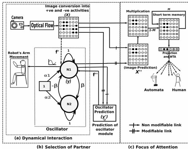
Figure 3: (a) Dynamical Interaction model (b) Selection of Partner: select a interacting partner on the basis of synchrony detection. (c) Shows attentional mechanism architecture.
