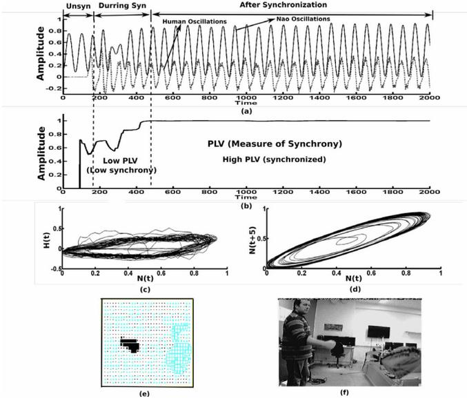
Figure 2: (a) Shows two motion signals (human and Nao). (b) PLV measurement. (c) Lissajous curve between  $N(t)$  (Nao's oscillation) and  $H(t)$  (Human's movements), (d) Lissajous curve between  $N(t)$  and  $N(t+5)$ . (e) Positive and Negative activities deduced from optical flow. (f) Real image seen by camera.
