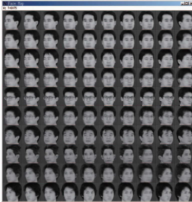
Figure 4: A map of facial images generated by a SOM 2 . Each row represents a child map, whereas each column represents a fiber of the SOM 2 .
